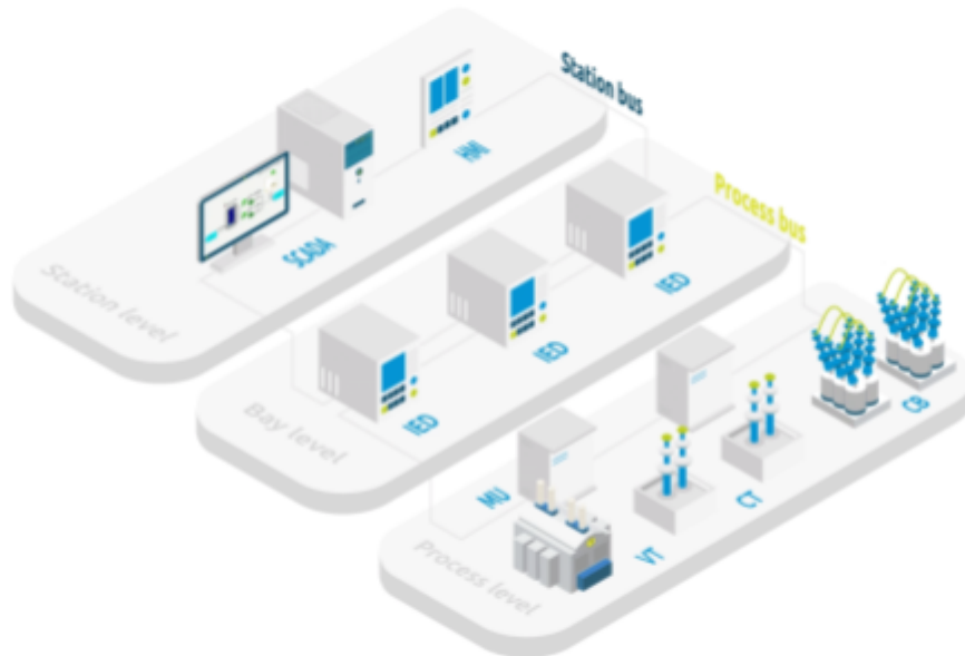
Figure 3: A sketch showing the arrangement of devices within an IEC 61850 substation(Credit: SGRwin)
