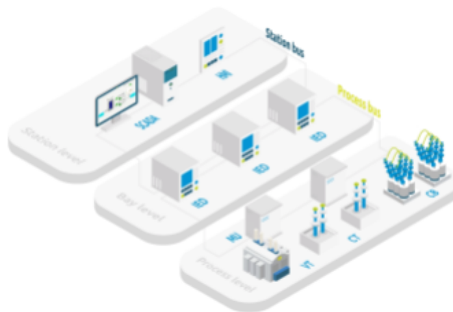
Figure 3: A sketch showing the arrangement of devices within an IEC 61850 substation(Credit: SGRwin)
